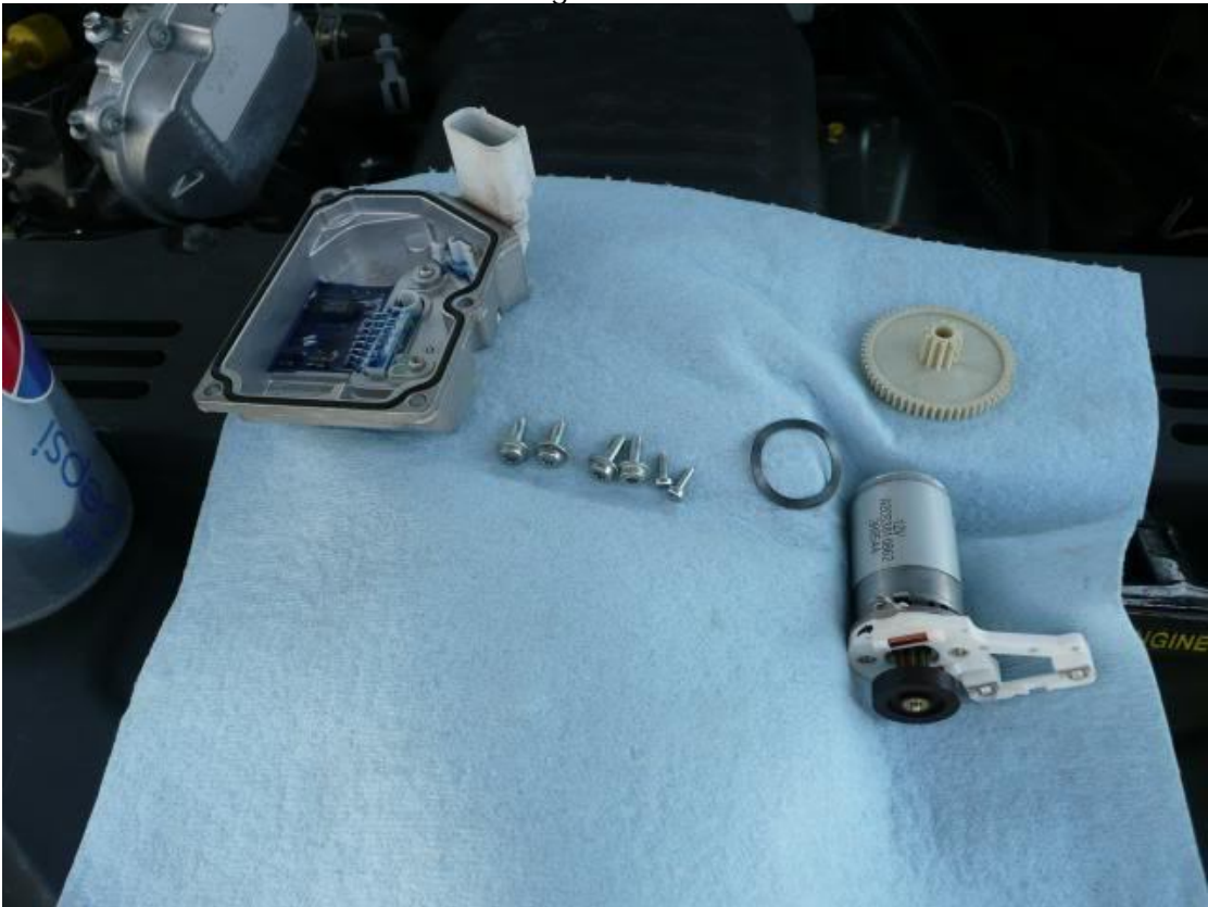
Here is the motor unit removed. NOTE the wave washer that is behind the motor. It goes back in the hole before installation of the motor again. The motor screws are T-10.
