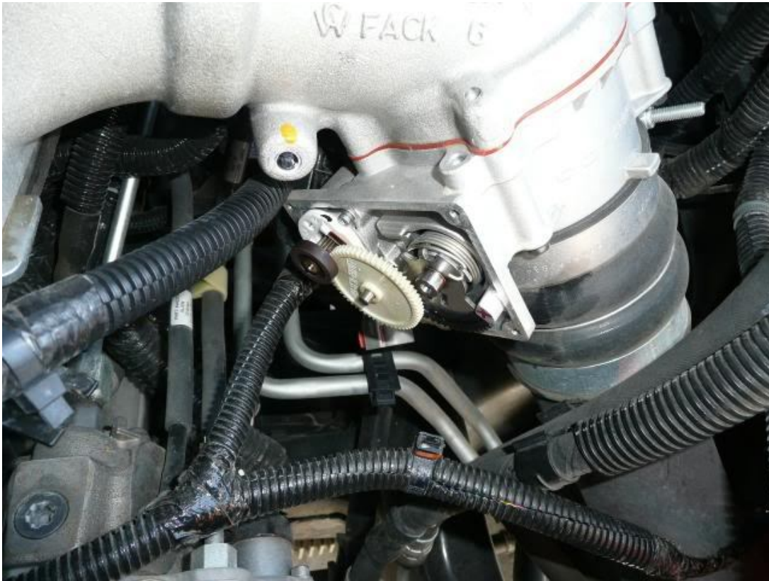
Here is the motor unit removed. NOTE the wave washer that is behind the motor. It goes back in the hole before installation of the motor again. The motor screws are T-10.
